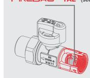
The valves have a FIREBAG® thermal safety device built into the steel inlet fitting. This solution makes it possible to leave the valve dimensions unchanged. FIREBAG® complies with the requirements of the DIN 3586 standard and activates at a temperature of 100°C-5K and withstands up to 650°C for 30 minutes at a pressure of 5 bar.
