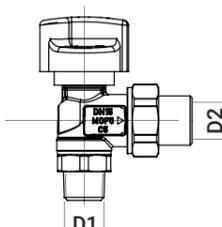
G2 straight valve with FIREBAG®, threaded version for gas appliances and hoses
