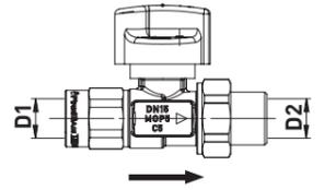
G2 90° valve with FIREBAG®, threaded/threaded fitting version for gas appliances
