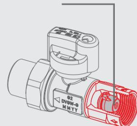
The valves have a FIREBAG® thermal safety device built into the steel inlet fitting. This solution makes it possible to leave the valve dimensions unchanged. FIREBAG® complies with the requirements of the DIN 3586 standard and activates at a temperature of 100°C-5K and withstands up to 650°C for 30 minutes at a pressure of 5 bar.
