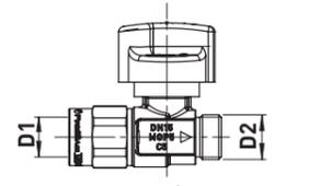
G2 90° valve with FIREBAG®, threaded version for gas appliances and hoses
